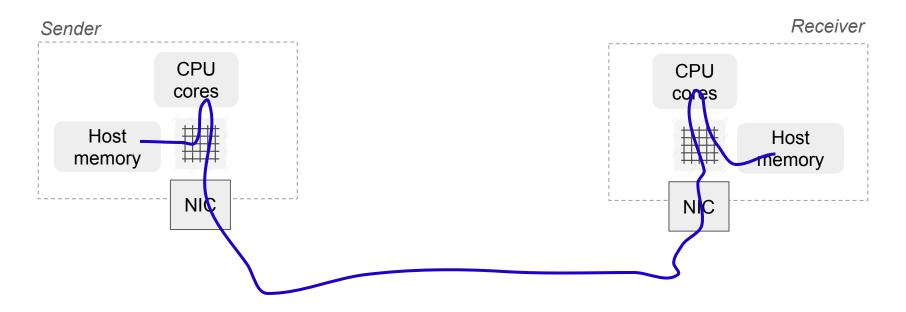
CPU is involved in moving data between memory and the NIC at both the sender and receiver
