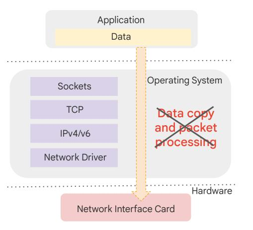
Goal: An application at server A can access data directly from the memory at server B without consuming (much) CPU time at server A or B.
