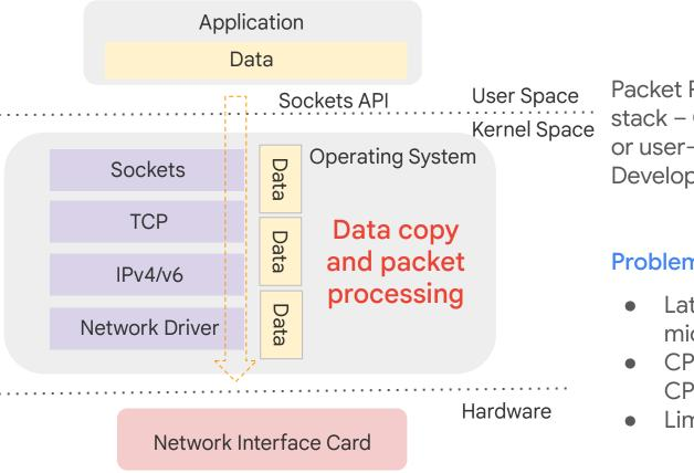
Packet Processing in host networking stack – Operating System (Linux, BSD) or user-space stacks (Snap, Data Plane Development Kit).
