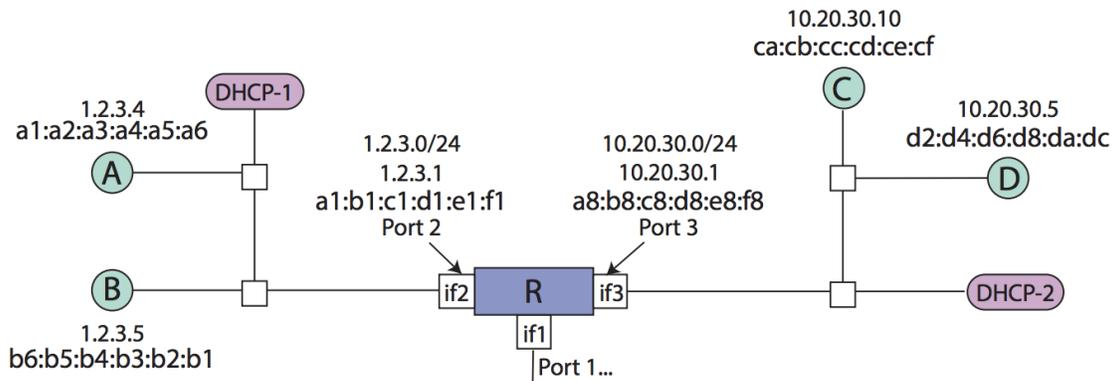
Consider the above topology. Here, two networks are connected through router R. R has three interfaces, each associated with a port, MAC address, IP address, and subnet.
