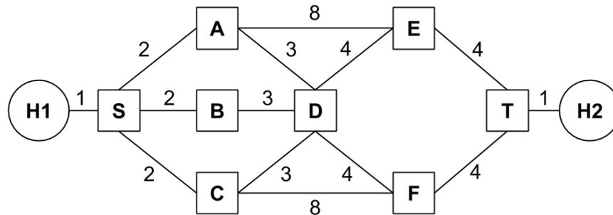
Suppose we have an L3 network with the topology shown above, and the routing algorithm used is link state.
