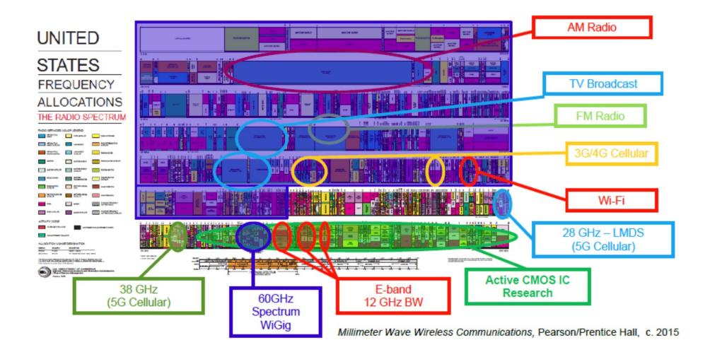
All existing commercial systems fit into a small fraction of the mmWave band Credit: Andrea Goldsmith CS 168, UC Berkeley: 55
